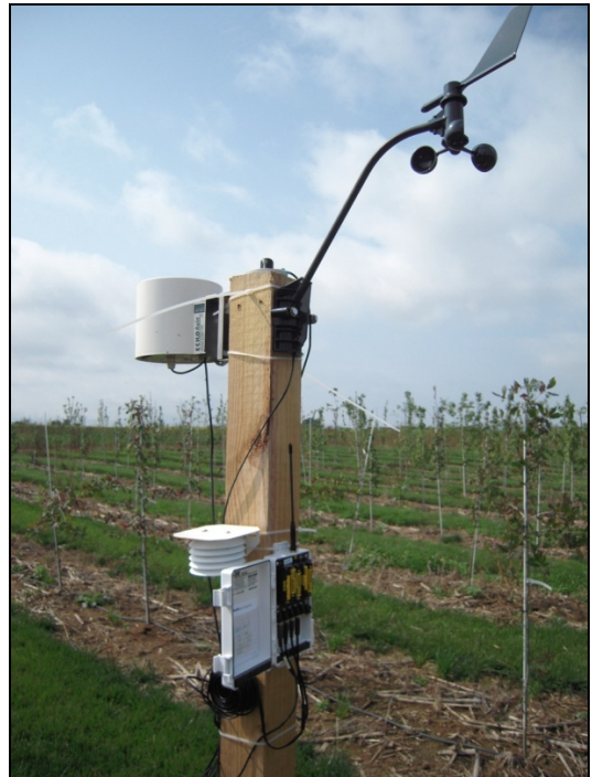
Fig. 1. Weather station wireless node in the field, with (from top), an anemometer (wind speed and direction); light sensor (measuring photosynthetically active radiation, PAR), rain gauge (rainfall); air temperature and relative humidity; leaf wetness sensor (dew) with a wireless radio node (open white box) which logs and transmits data at a specified time period (typically every 5 minutes).
