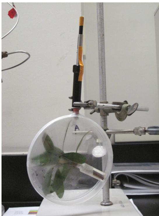
**Figure 1.** Modified Petri dish for headspace extraction of volatile chemicals using SPME.
