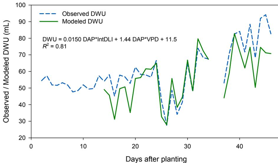
Fig. 3. Observed daily water use and the integrated model DWU of snapdragon ‘Opus Fresh White’ grown in perlite bag in a hydroponic system over 48 days. The model was based on the effect of days after planting (DAP), canopy intercepted daily light integral (IntDLI), and vapor pressure deficit (VPD). The first 10 days of the model was not included, due to lack of IntDLI data.
