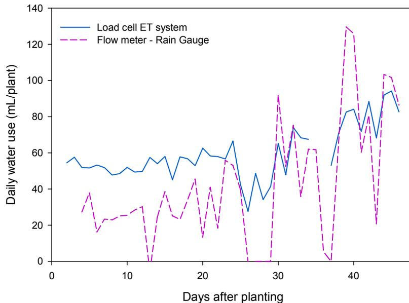
Fig. 1. Daily water use estimation of cut flower snapdragon production in a hydroponic system. A Load cell-based evapotranspiration measurement system and a water balance system using flow meter and rain gauges were compared. The lack of flow meter precision and occasional perlite clogging the rain gauges resulted in the lower reliability of the water balance system.
