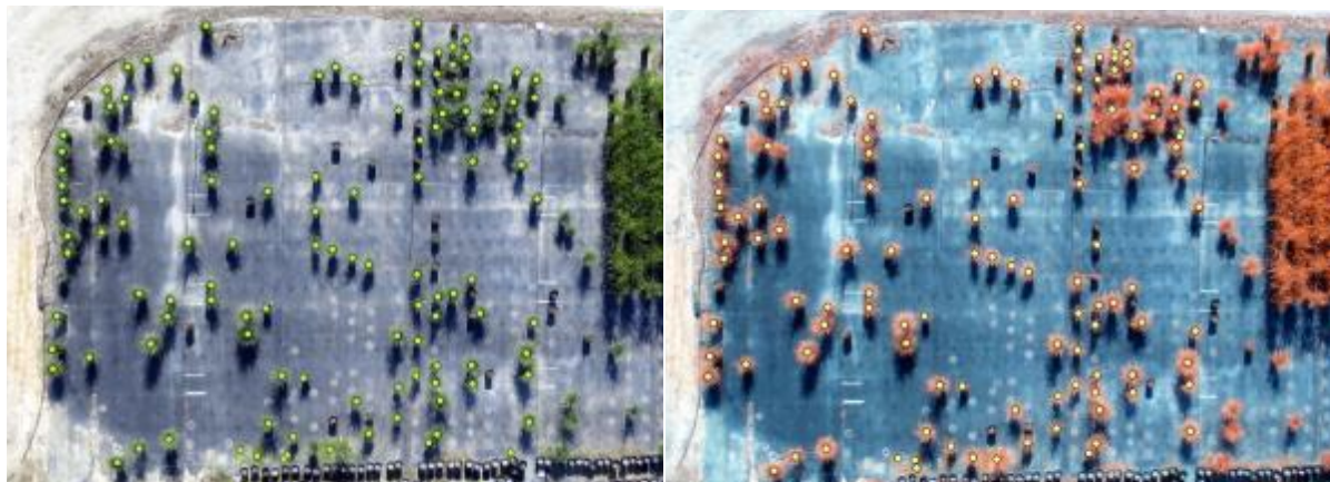
Fig. 2. Output image for a 'normal' (left) and NIR (right) image of the Miscanthus section. An option in Feature Analyst is for the software to place a visual mark (yellow dot in this example) on every object counted.
