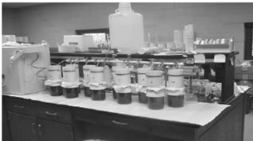
**Figure 1.** Experimental setup of soil columns and water application device.
