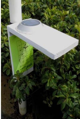
Figure 4. Insect monitoring station with solar lantern fixture.
