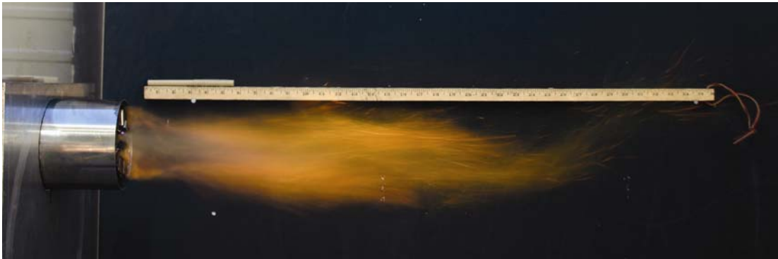
Figure 1. Flame produced from combustion of LBF in the retrofit NTG boiler.
