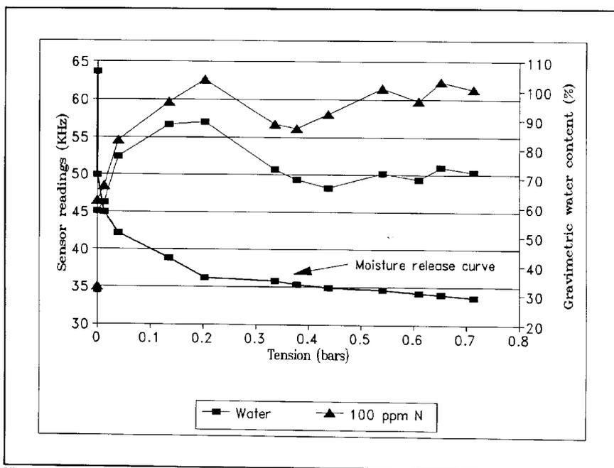
Figure 1. Response of moisture sensors in a 2 pine bark - 1 Canadian peat - 1 sand medium (by volume) initially saturated with water or 100 ppm nitrogen ( $\text{NH}_4\text{NO}_3$ ) solution.
