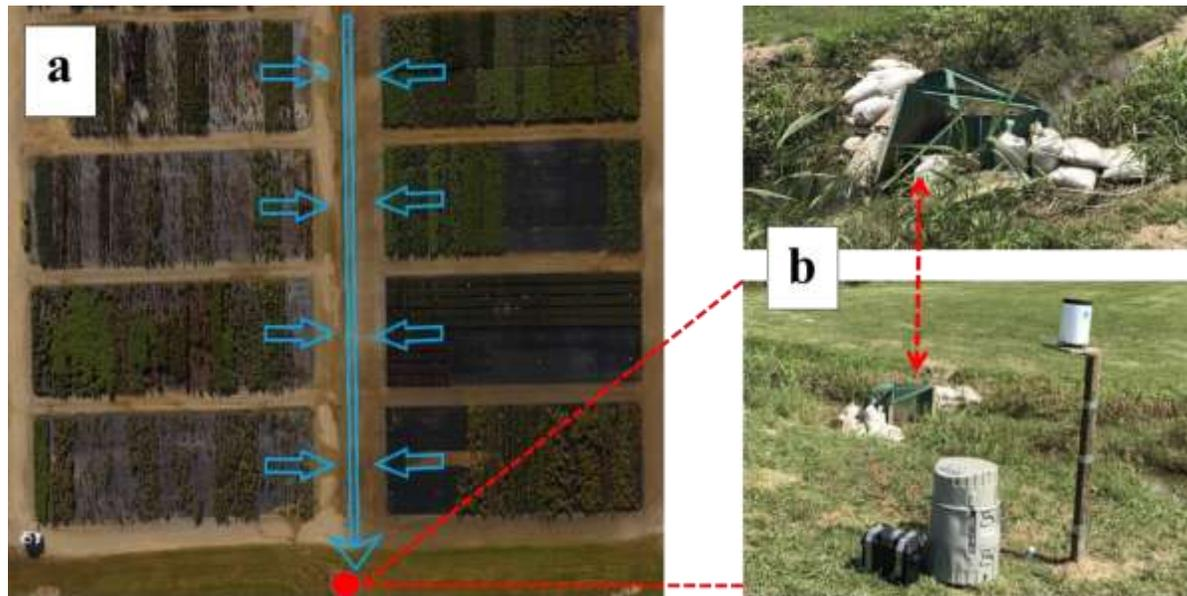
Figure 1. Location of (a) container pads and monitoring site outlet (filled red circle) and (b) H flume (top), automatic sampler and rain gage (bottom).
