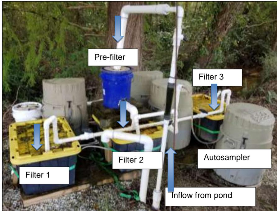
Figure 1. Pilot scale filters ( $n = 3$ ) evaluated with regard to phosphorus removal efficacy from irrigation runoff. Three iron oxide filters were automatically monitored over 7 weeks.
