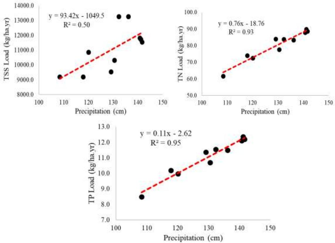
Figure 2. Relationship between annual precipitation depth and pollutants loads. TSS=total suspended solids, TN=total nitrogen, TP=total phosphorous.
