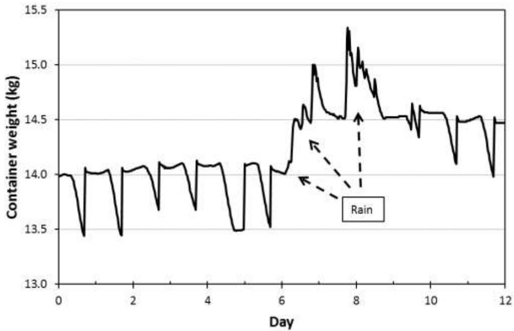
Fig. 5. Container weight (kg) of one trade 7-gallon (14-inch) Podocarpus plant recorded every 30 minutes for 1-12 December 2017 at the University of Florida, Gainesville.
