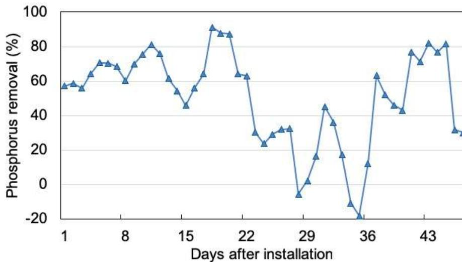
Figure 2. Phosphorus removal efficacy (3-day moving average) of a passive flow iron oxide filter ( $n = 3$ ) installed at a SC nursery.
