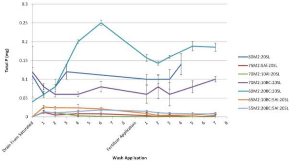
Figure 2. The effects of biochar and alumina on the leaching of dissolved phosphorus from each substrate containing base green roof media (M2), SmartLeaf® compost (SL), mushroom compost (Mu), alumina (Al), and/or biochar (BC).
