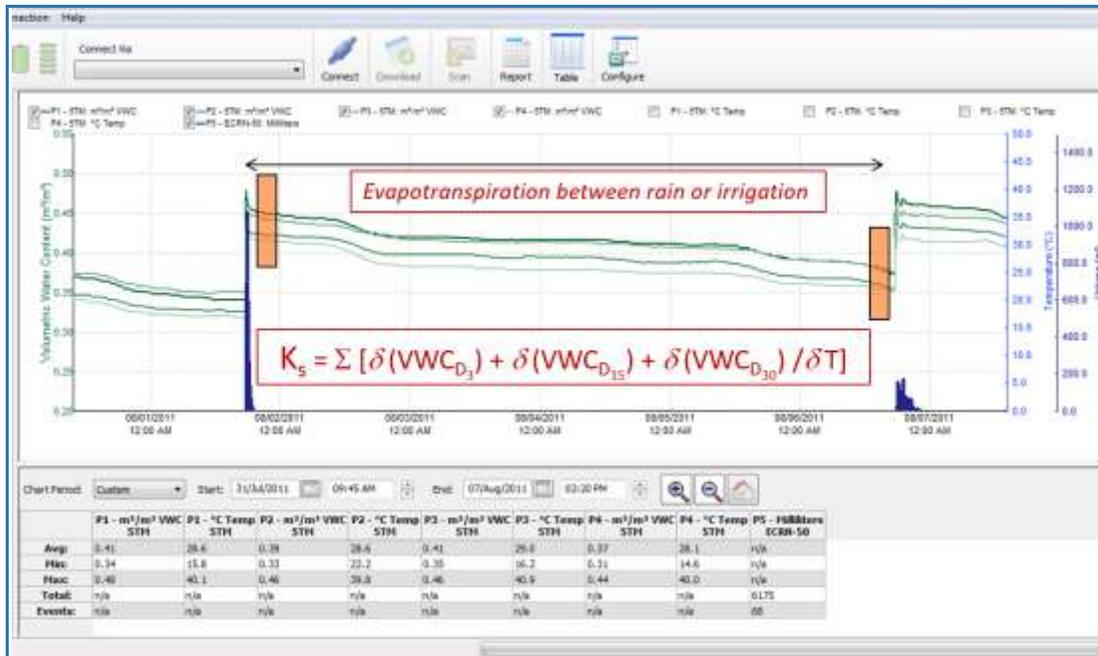
Figure3. Estimating average daily water loss ( $K_s$ ) values from soil moisture data at three depths (3 cm, 15 cm and 30 cm), between rain or irrigation events.
