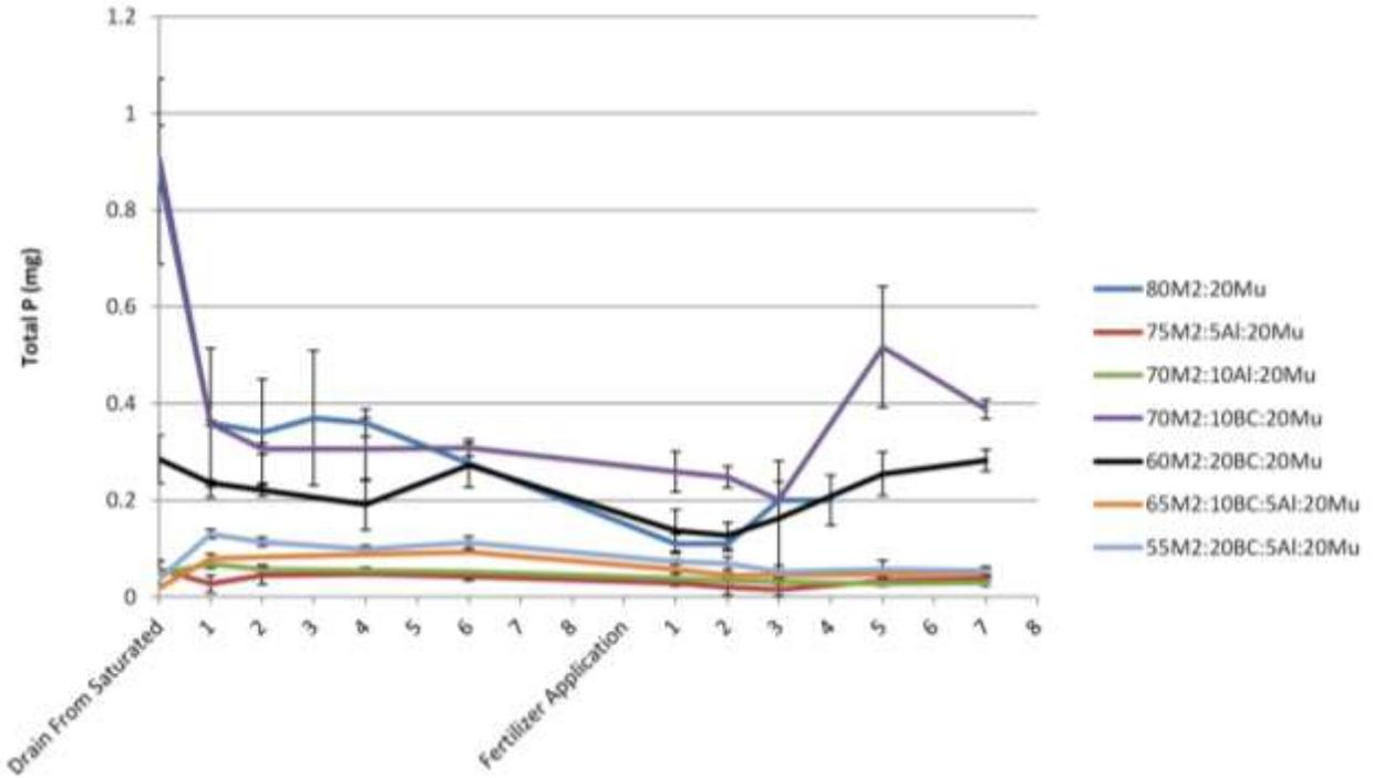
Figure 1. The effects of biochar and alumina on the leaching of dissolved-phosphorus from each substrate containing base green roof media (M2), mushroom compost (Mu), alumina (Al), and/or biochar (BC).
