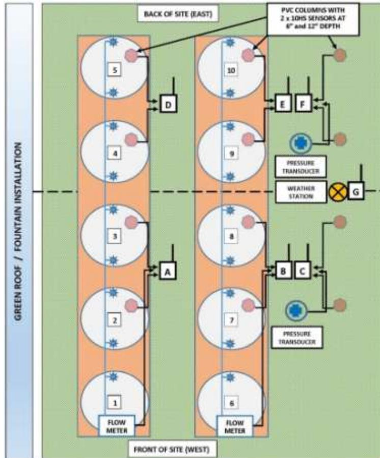
Figure 2. Site Installation diagram of the sensor network: Pink hexagonal icons indicate soil sensor locations in numbered bald cypress trees and four positions within the zoysia grass area. Letters within squares indicate EM50R radio dataloggers. Other sensors noted in annotated boxes.
