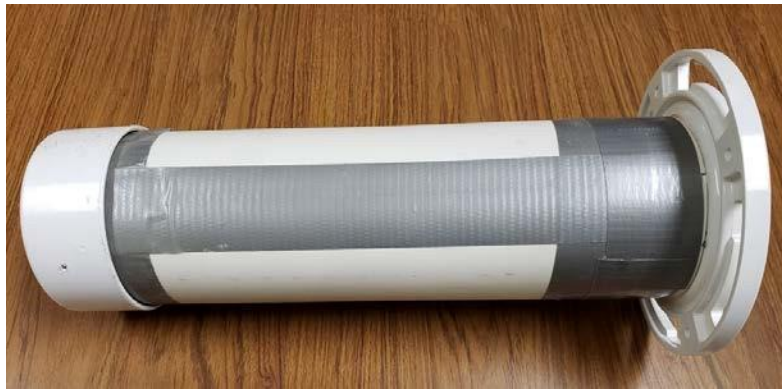
Figure 1. A lysimeter constructed from 4 inch PVC and used to evaluate glyphosate leaching in two substrates.
